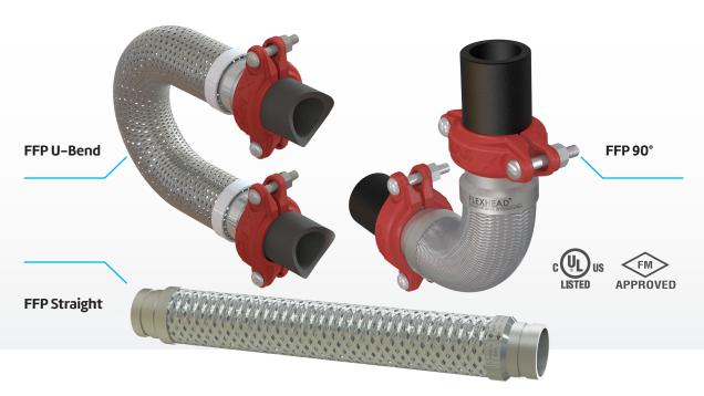
Flexhead® Flexible Pipe (FFP) products are stainless steel hoses and available with SLT coupling connections. Available in lengths of 24" (bends up to 90°) and 48" (bends up to 180°) with OD of 2", 2 ½", 3" and 4". Pressure rating for 2", 2 ½", and 3" is 300PSI and 4" at 250PSI. An easy, cost effective, and a quickway to connect pipes at odd angles or to reduce the number of couplings and fittings required.
